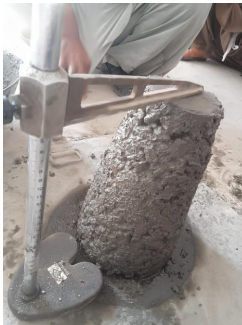
Figure 1: Measuring the workability of a fresh BLA concrete specimen using the slump cone test
