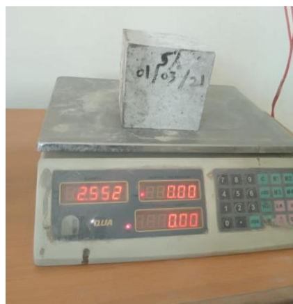
Figure 3: Specimen being weighed prior to testing
