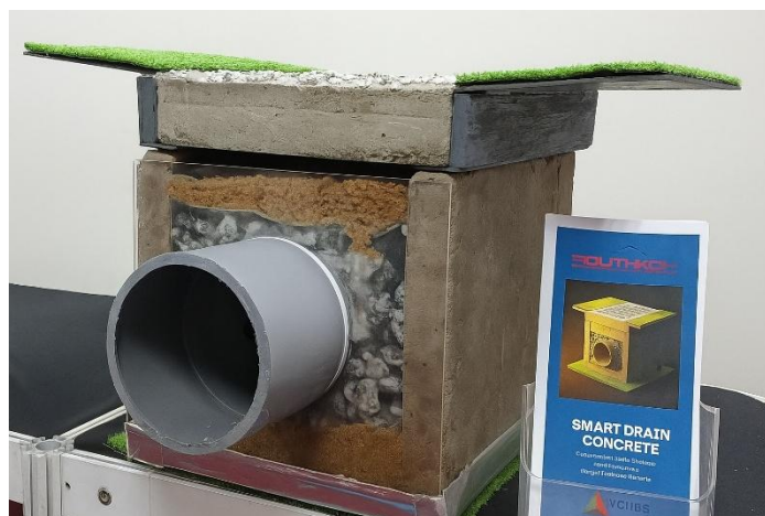
Figure 5 : Prototype of Smart Drain Concrete
